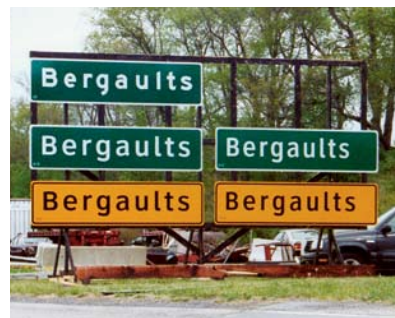
19 On display at the Penn State test track: Highway Gothic, top left, and Clearview, middle and bottom.
